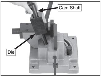
Figure 10. Lifting clamp cam shaft and die.
